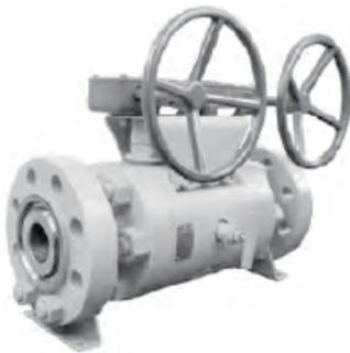
Neway supplies DBB compact manifold ball valves which are equipped with two balls in one body. The series can be designed in three-piece, long or customized pattern to satisfy the different installation requirements. DBB compact manifold ball valve design reduces the weight and space compared with installing two conventional valves when it achieves safer application. These valves are usually applied in marine and offshore industry.
