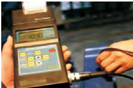
Paint Thickness Test
