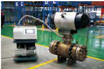
Low Fugitive Emission Test
