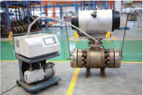
Low Fugitive Emission Test
